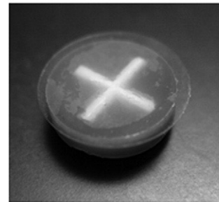
Fig. 1. Adult neurons were cultured on 15 mm 2 glass cover slips and supported in the respiration chamber by a silicone-topped teflon stir bar. (A) Neurons prepared from middle-age rats cultured on a glass cover slip. (B) Neurons prepared from old rats cultured on a glass cover slip. The fields pictured are 0.04 mm 2 . (C) Silicone-topped teflon stir bar designed to support substrate-adherent neurons on a 15 -mm glass culture slip while measuring oxygen consumption.
